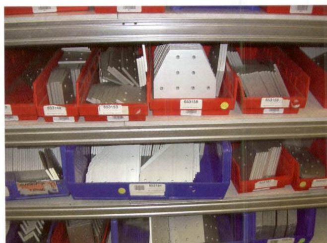
Figure 14. TSLOT joining plate bins in the accessory storage room.
