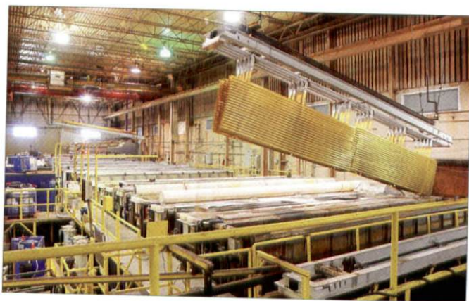
Figure 8. Anodized extrusions coming out of the anodizing tank.
