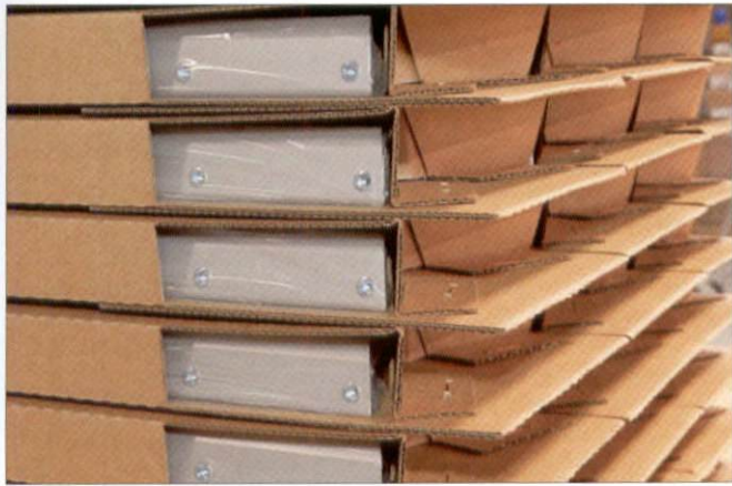
Figure 10. Customized packaging of fabricated extrusions with plastic and paper sleeving, separating fabricated product.
