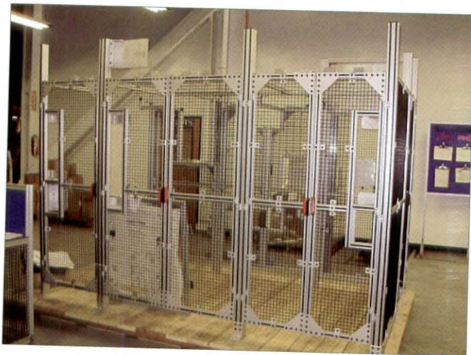
Figure 9. A specialized enclosure assembled at Futura prior to packaging and shipping, utilizing their TSLOT extrusions and attachments.
