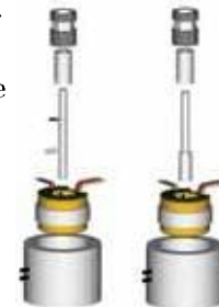
Spring pin/retaining ring method (left); shoulder/adhesive method (right)
